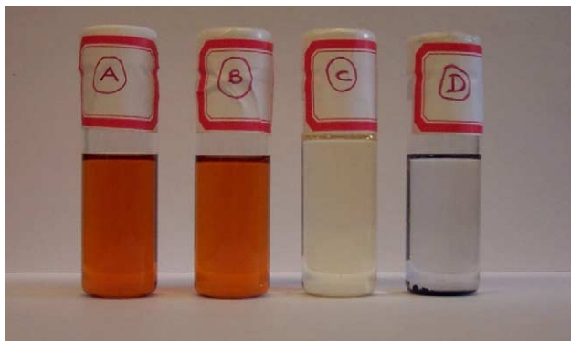
Fig. 6. Photograph of solution samples in benzene/methanol mixture: (A) MMA-6.0%MAA/PbS (1 day); (B) untitrated MMA-6.0%MAA/PbS (15 days); (C) titrated MMA-6.0%MAA/PbS; (D) usual bulk PbS powder.
